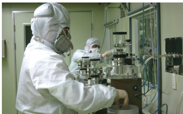
Equipment for an inhalation toxicity test
